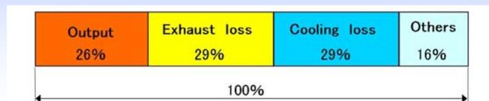
Fig. 2 Example of heat balance in a conventional engine
