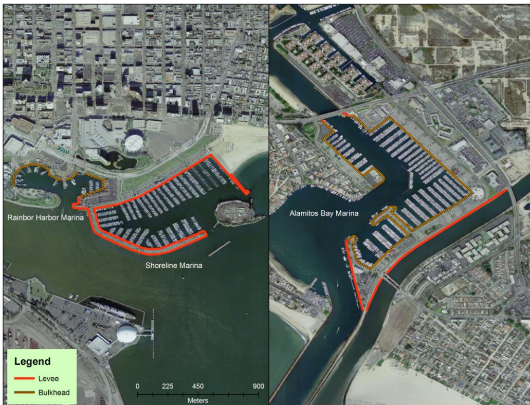
Figure 6. Existing Protective Coverage at Long Beach's Marinas
